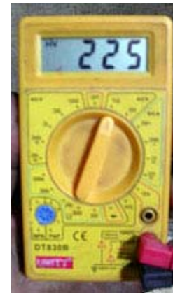
Figure 8: The WLED lamps are power by 225 AC in the village.
